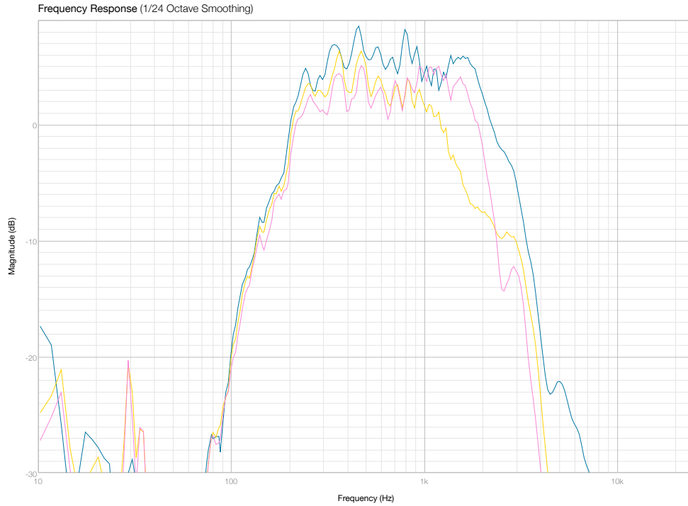
Midwoofer Horizontal Off-Axis Frequency Response at 1 Meter with Crossovers, On Axis (Blue), 30 Degree (Pink) 60 Degree (Yellow)
