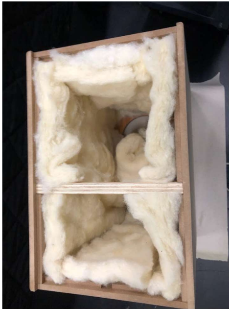
Figure 31 - wool inserted into mid/high cabinet
