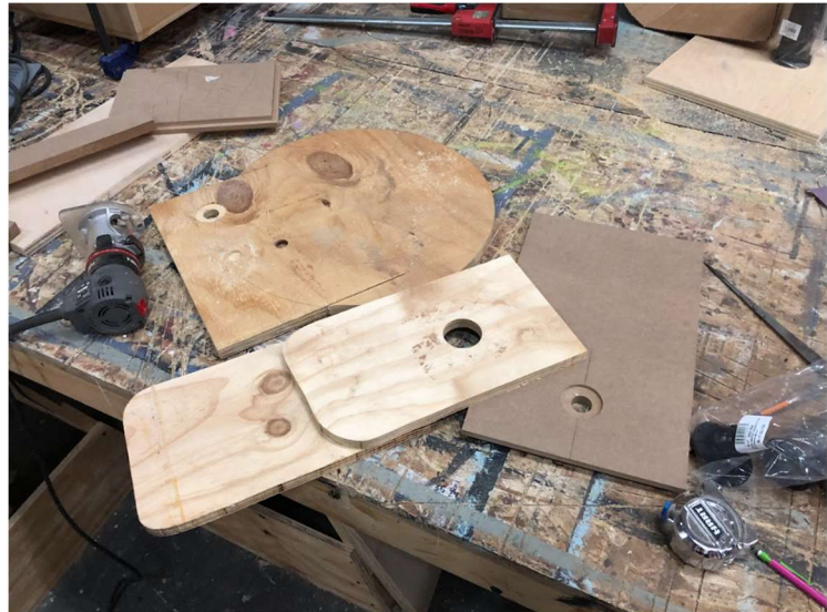
Figure 23 - custom jig used to ensure uniform cuts
