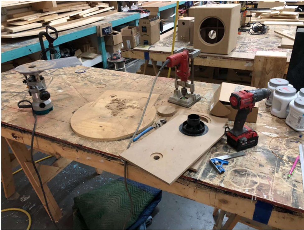
Figure 24 - set up for cutting port holes
