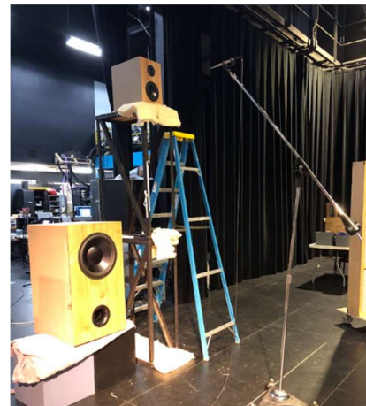
Figure 34 - mid/high being tested on a tall stand, wool used to eliminate reflections from the stand
