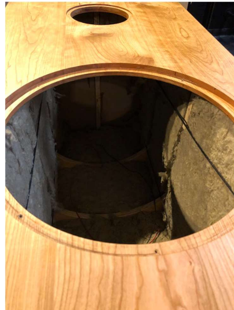
Figure 30 - rock wool inserted into subwoofer, held in place via tie-line
