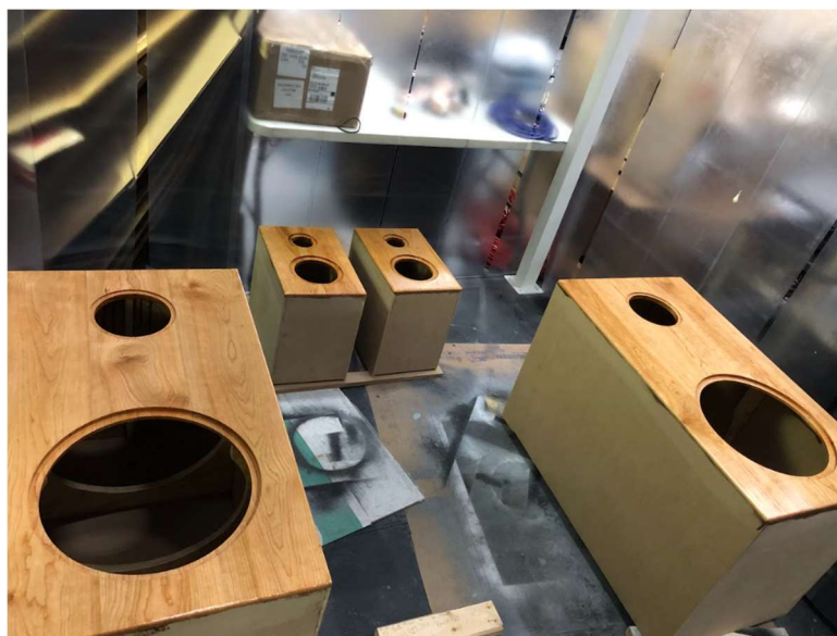
Figure 29 - cabinets drying after first coat of finish
