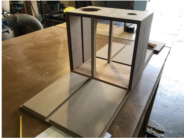
Figure 28 - dry fitting of mid/high cabinet
