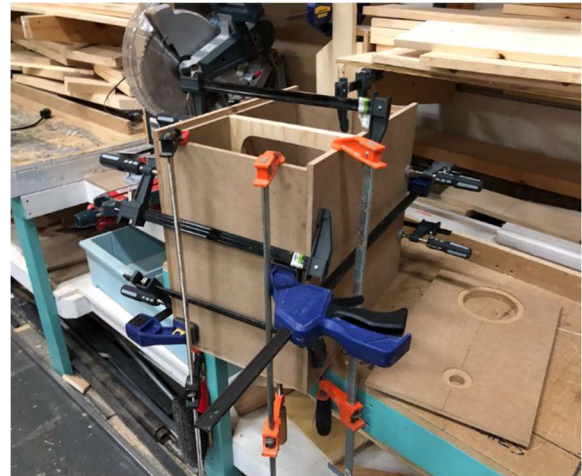
Figure 27 - clamping down mid/high cabinet while glue dries
