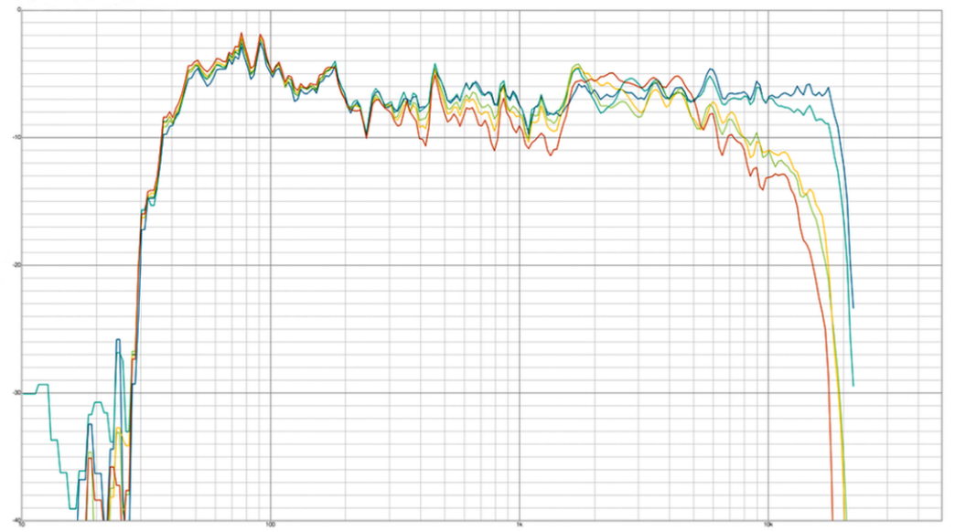
FREQUENCY RESPONSE WITH HORIZONTAL OFF-AXIS (1/24TH OCTAVE SMOOTHING)
